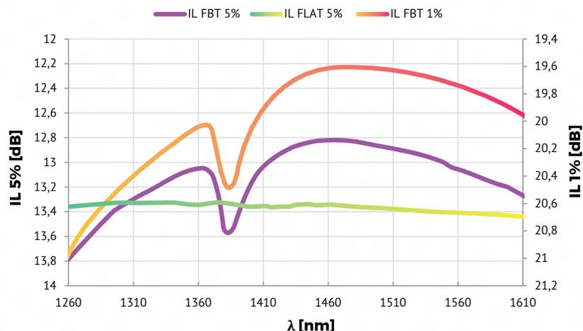
Figure 4. Characteristics of monitoring ports manufactured in the FBT and flattened technologies
