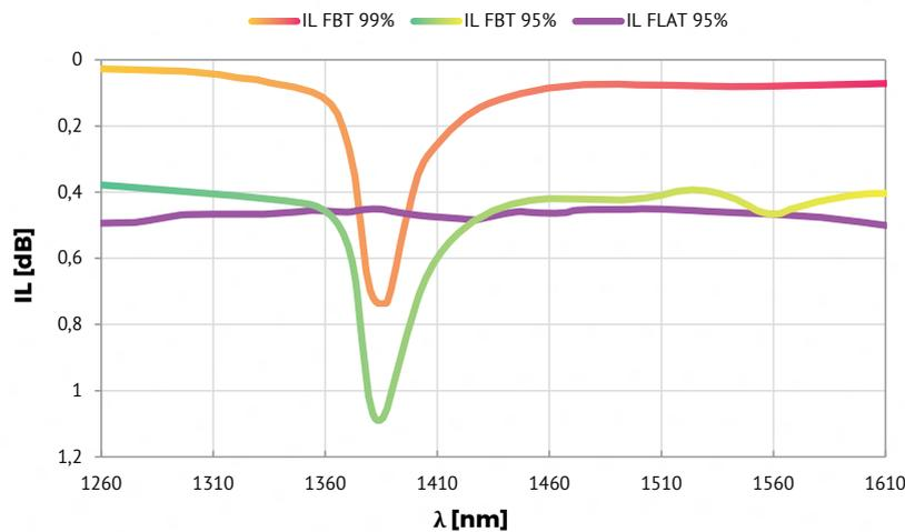
Figure 5. Characteristics of line ports manufactured in the FBT and flattened technologies
