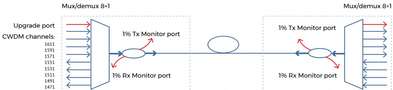
**Figure 2.** Bidirectional CWDM link with monitoring
