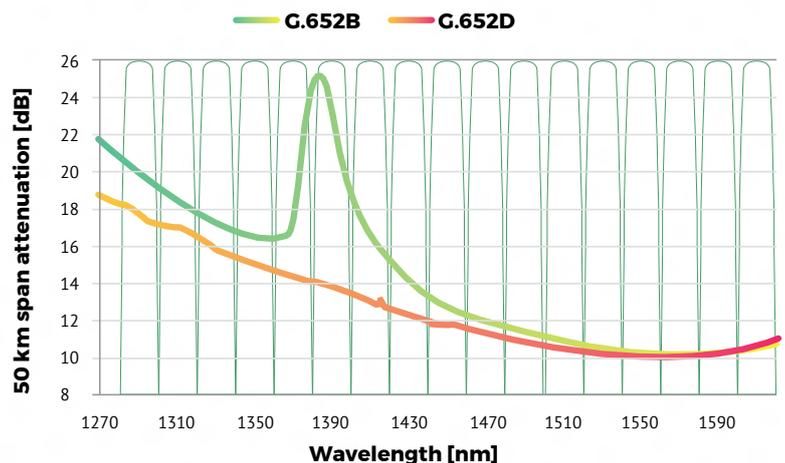
**Figure 1.** Spectral attenuation characteristics of 50 km G652B and G.652D fibers with schematically shown CWDM channel positions
