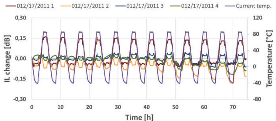
FIGURE 6 – Changes in insertion loss value for selected ports of Fibrain 1x8 splitter during testing in the environmental chamber
