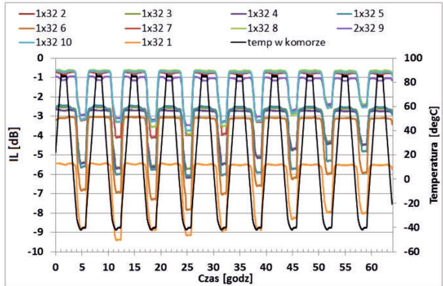
FIGURE 5 – Changes in insertion loss value for selected ports of AAA-branded 1x32 splitter during testing in the environmental chamber – fluctuations in attenuation value from 3 up to 9 dB
