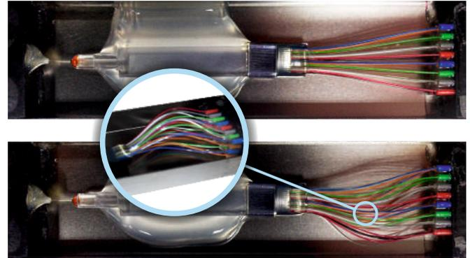
FIGURE 3 – Xyyyy-branded 1x32 splitter containing the correct amount of adhesive before (above) and after (below) testing in the environmental chamber. A receding fiber and macrobendings are evident.
