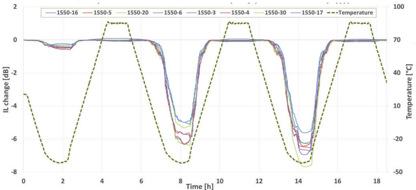
FIGURE 2 – A sample Xyyyy-branded 1x32 splitter vs. the environmental chamber – changes in attenuation by approx. 8 dB are evident.
