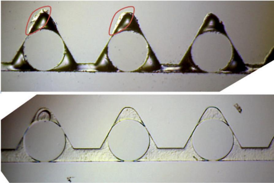
**FIGURE 7 – The influence of humidity on fiber array elements coming from various producers.**
